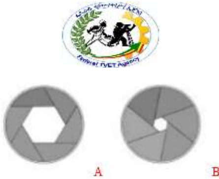
Fig. 3.6. A when diaphragm is opened to allow maximum light for high power objective B when diaphragm is closed to allow low light for lower power objective
