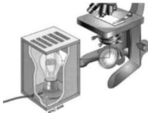
Fig. 3.7. Setting up a Lamp for a Microscope
